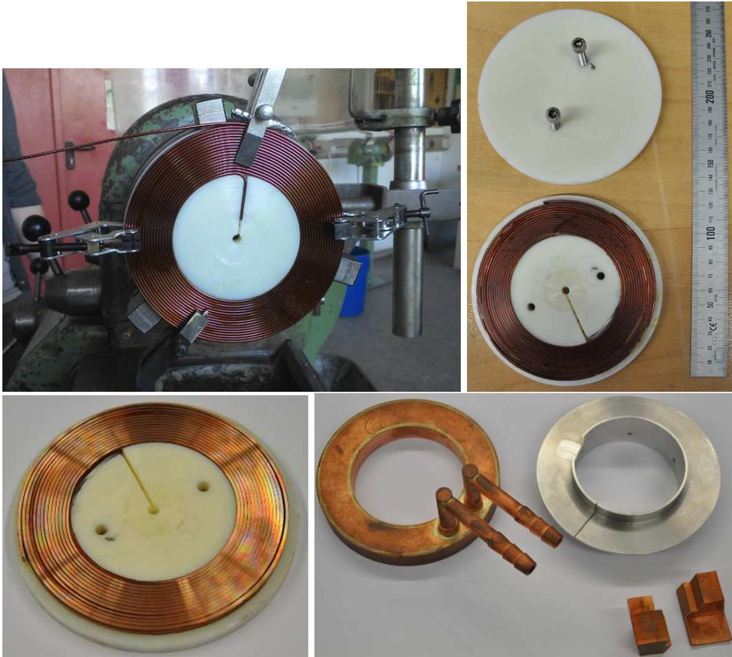
**Figure A.1.:** Manufacturing a coil.
